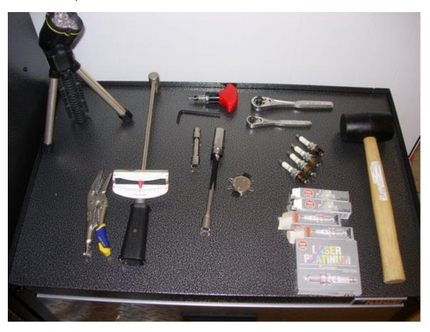
Start off by taping the spark plug socket to the medium-length extension with some electrical tape. This is good for ensuring the socket doesn't come off the extension when replacing the plugs. (If it gets stuck on the spark plug, you'll have to remove that plug and start over.)
