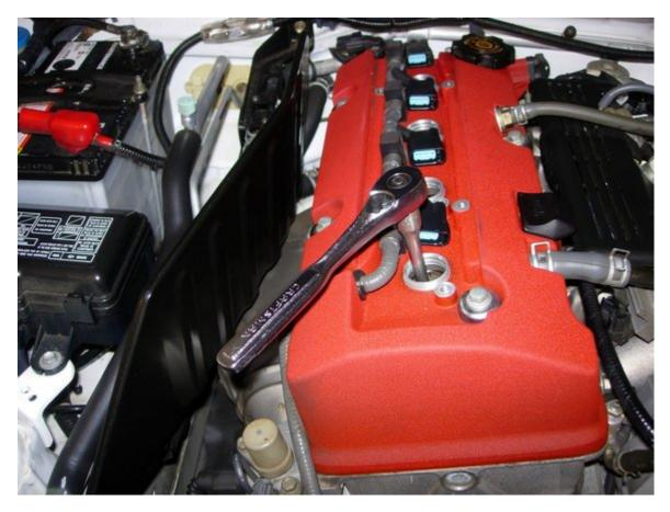
After you get a spark plug out, I replace that plug immediately with a new plug since you have all the tools at hand already. Before you insert your new plugs, confirm your gap again - Honda states: Standard (New): 1.0 - 1.1mm (0.039 - 0.043 in.).
