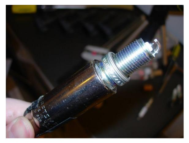
Now lower the plug into its cylinder. Be very careful about not crossthreading the hole! The best way to do this is to insert the plug, turn it counter-clockwise a half turn to ensure its flush, and then hand-tighten it clockwise. With 180° turns of the socket, it will take about 25 turns to get the spark plug snug. It should turn in pretty smoothly - never force a spark plug in!
