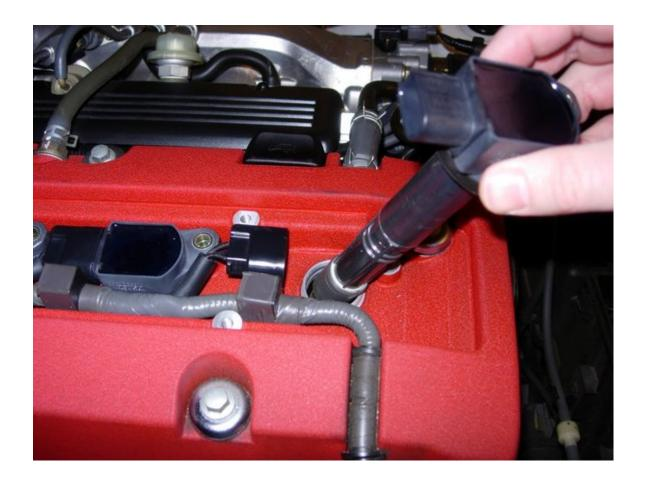
Now, use the 5/8" or 16mm spark plug socket on the medium length extension to remove the spark plug. Make sure you properly seat the socket on the plug - you don't want to break the plug off in the engine! Again you want to "snap" the plug loose - make sure you have a good seat. A rubber mallet will be helpful to break the spark plug's seal against the engine - be careful of stripping the spark plug hex - you don't want to deal with a stripped spark plug!
