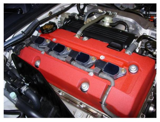
Next step is to remove the ignition coil retainer bolts. Use a 10mm socket on a short extension to unbolt each ignition coil (once again, "snap" them loose with a mallet and quick force), and pull to extract it from
